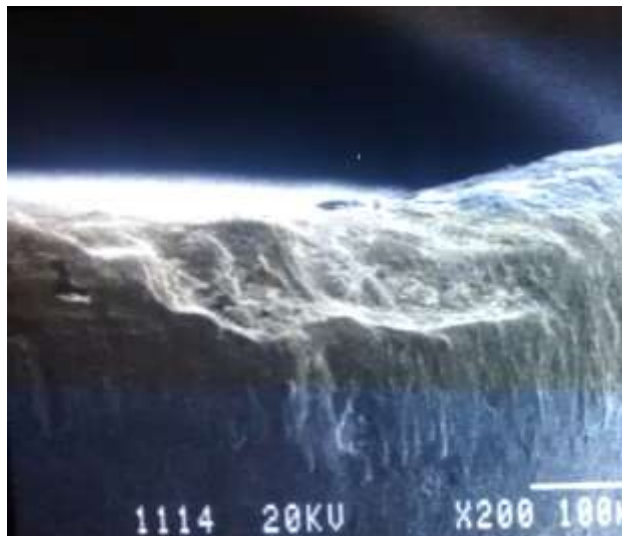
Fig.5 The cutting insert after 3minutes of machining at v=80m/min,f=.08mm/rev and W.H.=40HRc.
