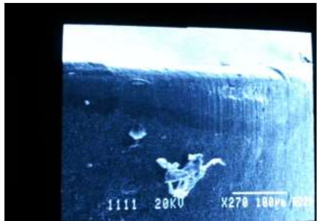
Fig.6 The cutting insert after 2minutes of machining at v=140m/min,f=.22mm/rev and W.H.=47HRc.
