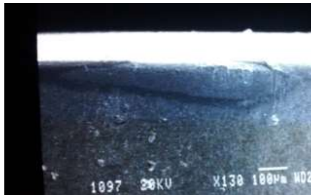
Fig.7 Edge Chipping of insert at v=200m/min, f=.22mm/rev and W.H.=54HRc
