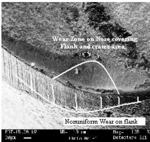
Fig.1 Coated carbide tool after 6min of machining at v=80m/min, f=0.08mm/rev and W.H=40HRC
